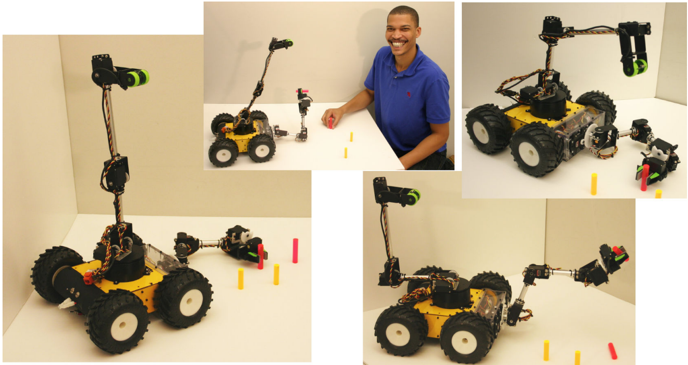
Figure 6: The Regis prototype posing with the second author. Note the variety of configurations of the “goose neck” webcam and “crab arm” manipulator with gripper.
